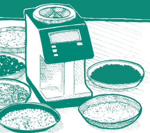
Testing seed using an electronic moisture meter
