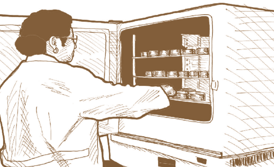
Figure 3.12 Moisture test. Drying the seeds in the oven (left) and placing the seed to cool in a desiccator (right)
